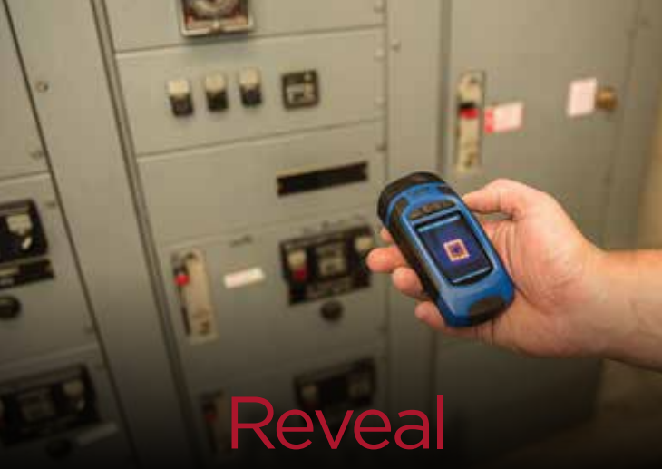
Handheld Thermal Camera with 32,136 Pixels
