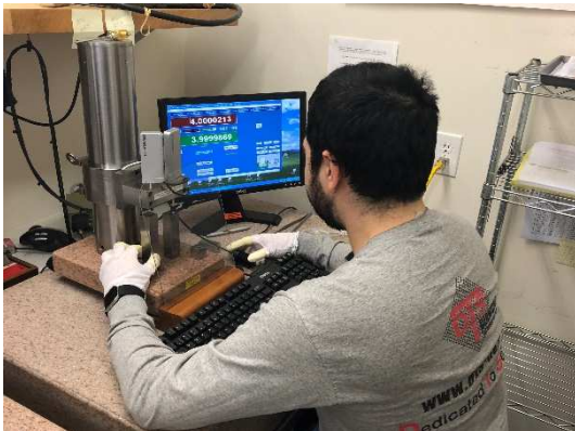
Gage block calibration_©DTS
